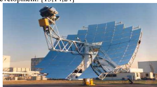
Figure (46): A parabolic solar collector concentrating the sun's rays on The solar cells (Solar Stirling Engine)
